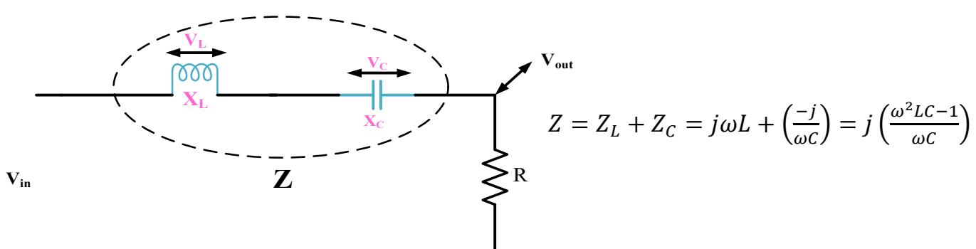
$$\begin{cases} \text{if } \omega \rightarrow \omega^2 LC - 1 < 0 \Rightarrow Z = R \\ \text{if } \omega \rightarrow \omega^2 LC - 1 > 0 \Rightarrow Z = \infty \\ \text{if } \omega = \omega_r \rightarrow \omega^2 LC - 1 = 0 \Rightarrow Z = R \rightarrow 0 \Rightarrow \omega_r = \frac{1}{\sqrt{LC}} \end{cases}$$
